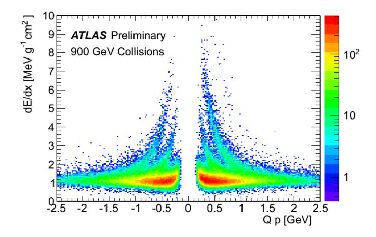
There are 80,000,000 pixels and 160,000 tracks. So this plot is not just telling us how well the dE/dx works, it's telling us how well cross-calibrated the pixels are.
