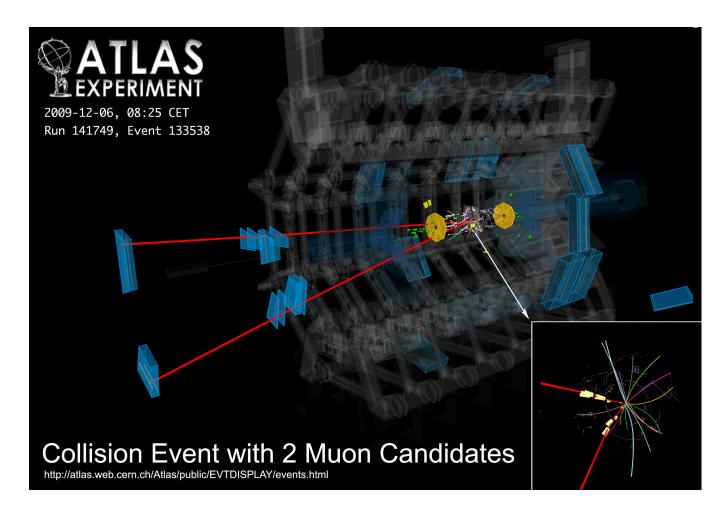
We have muons – but not many (dozens). In fact, we need to keep the toroids off in order to get a track in the muon spectrometer: otherwise they would be bent back into the calorimeters.
