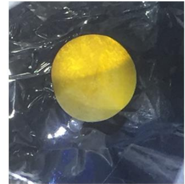
Target B – no thermal insulation (1" CCR). Thick cryo -condensed 'ice' layer visible on the reflector surface
