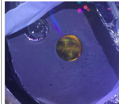
Target D – thermally insulated (0.5"CCR + \Phi 4mm S-LAH79 ball). No condensation visible
