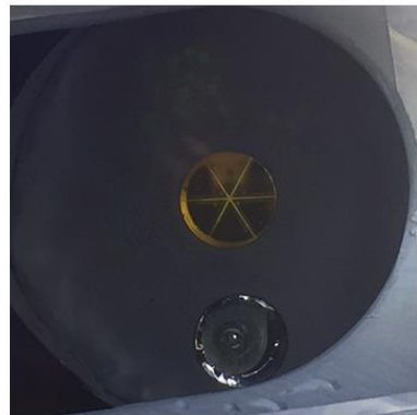
Target E – thermally insulated (0.5"CCR + \Phi 4mm S-LAH79 ball). No condensation visible
