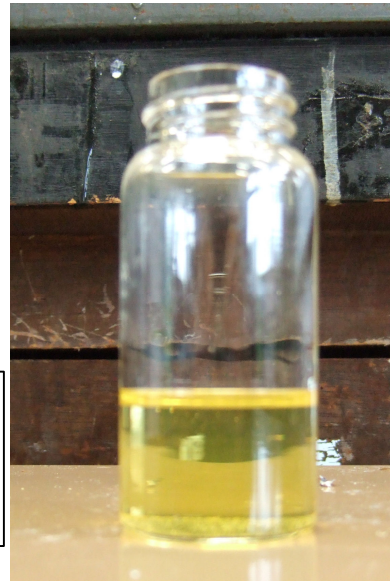
Newly developed CE resins for HF accelerator magnets
