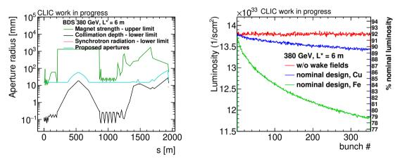
▶ Using steel leads to high sensitivity to the effect; luminosity decays rapidly along the bunch train
