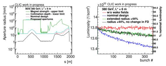
Extending apertures by 44% reduces sensitivity to resistive wall effect by a factor of 3
