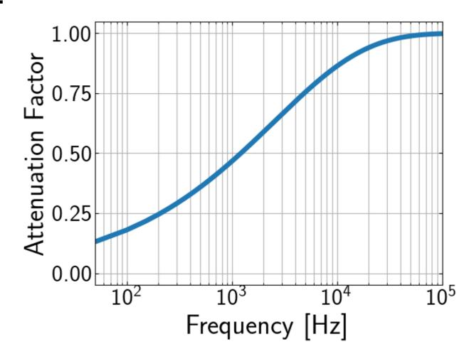
$$B(d) = B_0 \exp\left(-\frac{d}{\delta}\right) \qquad \delta = \sqrt{\frac{2}{\omega\mu\sigma}}$$
