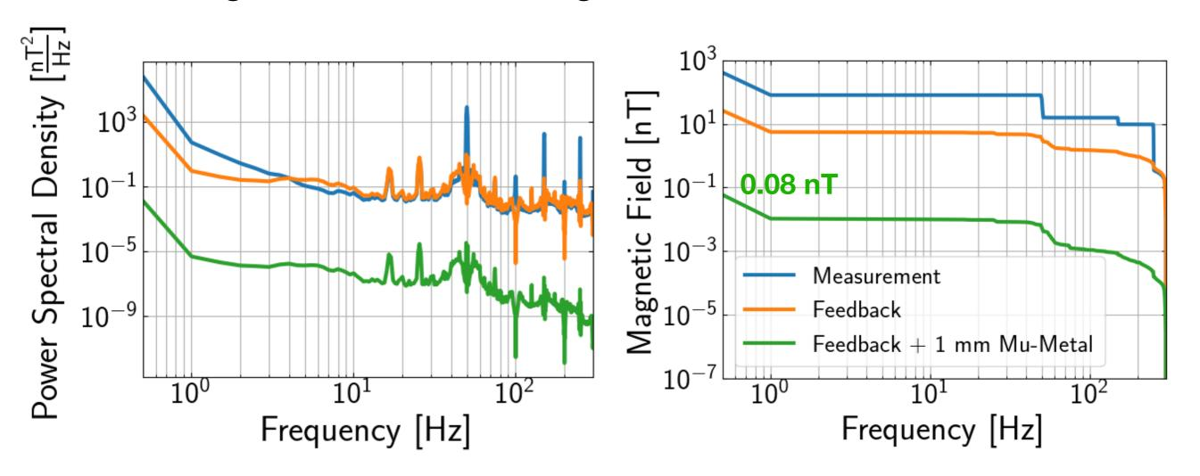
A 1 mm mu-metal shield brings field within tolerance.
