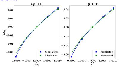
Shift in vertical tune from changing strength of the two quadrupoles in SuperKEKB HER closest to the IP. Measured and simulated values. Lines are made by fitting  $\beta_{average}$ .
