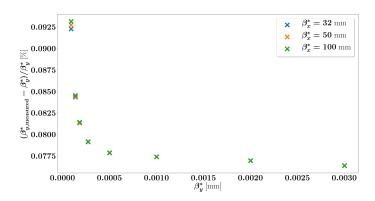
▶ Error in measurements due to different  $\beta_y^*$  and  $\beta_x^*$ .
