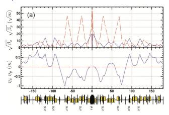
➤ Two sections with sextupoles for correcting the vertical and horizontal chromaticity separately. Likewise downstream.
