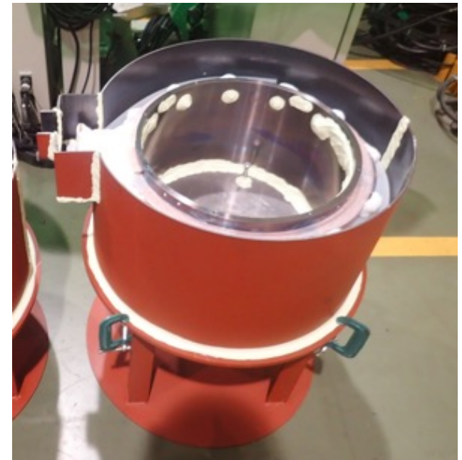
Preparation for Resin Molding
