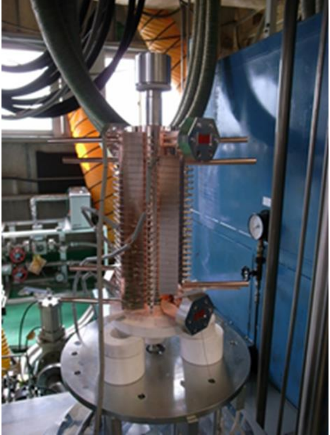
Brazing tuning pin and water cooling
