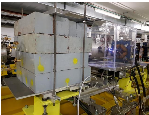
Provisional Beam dump
