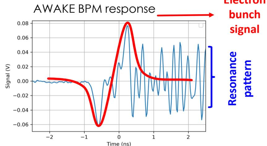
Measuring using the **present system** is problematic due to pickup resonances in the GHz range excited by the beam
