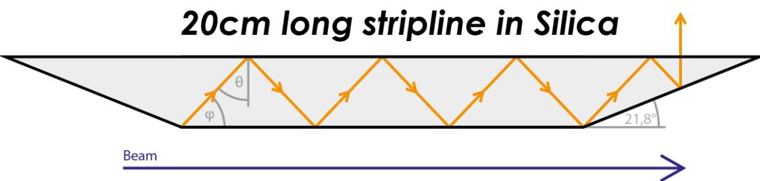
Investigating **long(er) radiator** (mm to 10s of cm) in order to increase the light yield and use those for **low(er) beam energies** and at **large distances** (few cm) from beams
