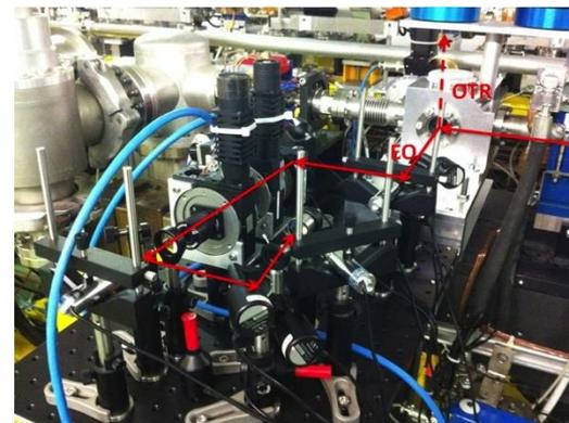
Crystal chamber (4mm ZnTe), crossed polariser
