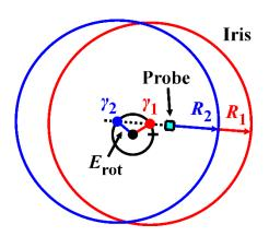
$$E_{\text{rot}} = \frac{R_1 - R_2}{2\sin\left(\frac{\gamma_2 - \gamma_1}{2}\right)}$$
