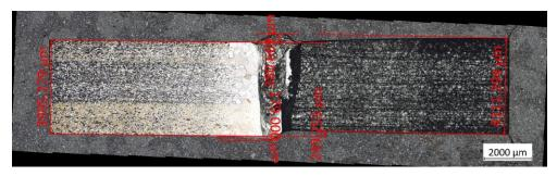
The beam is focused on the Nb to compensate for the lower energy required to melt NbTi
