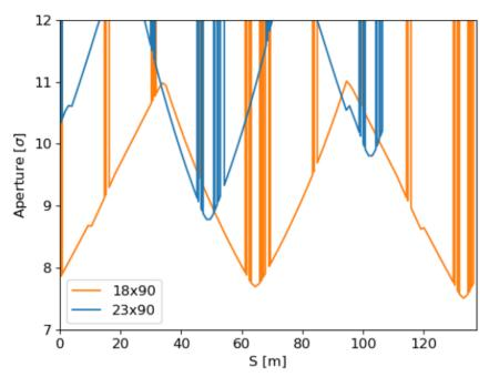
HE-LHC injection aperture in the arc for two optics options. Courtesy HE-LHC design team
