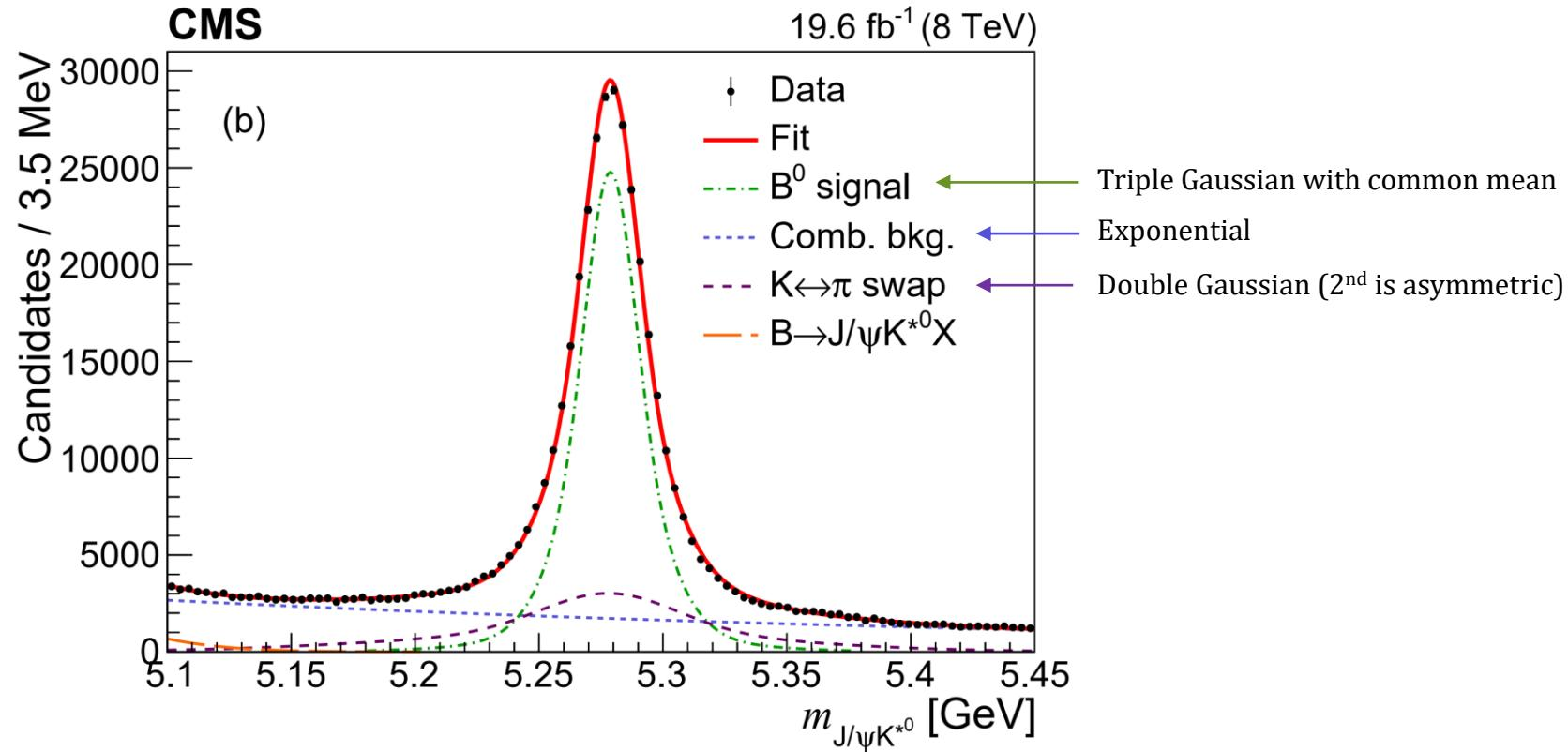
The resolution parameters and the shape of  $K \leftrightarrow \pi$  swapped component are fixed from simulation (see backup)
