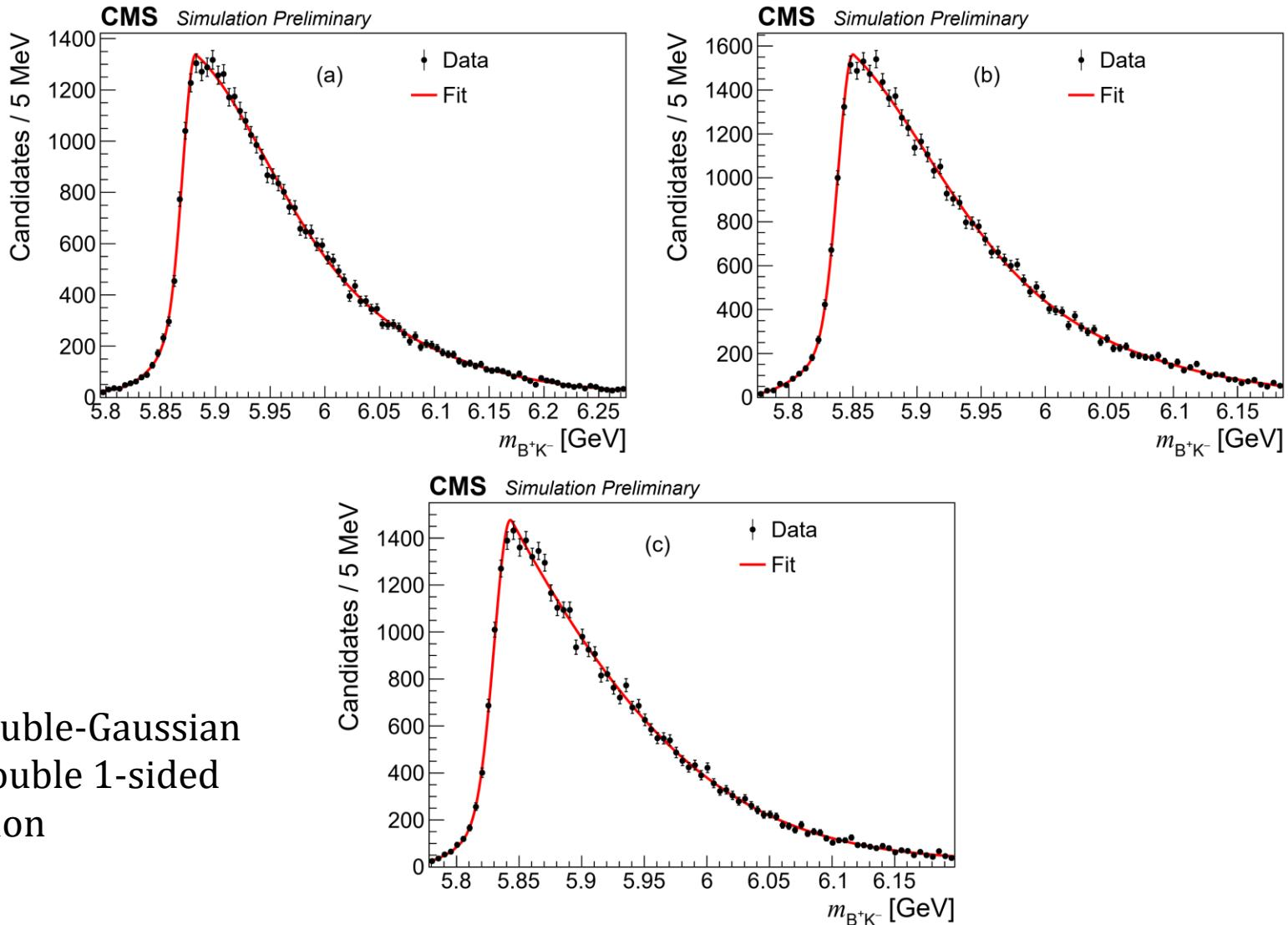
Product of a double-Gaussian function and double 1-sided Gaussian function
