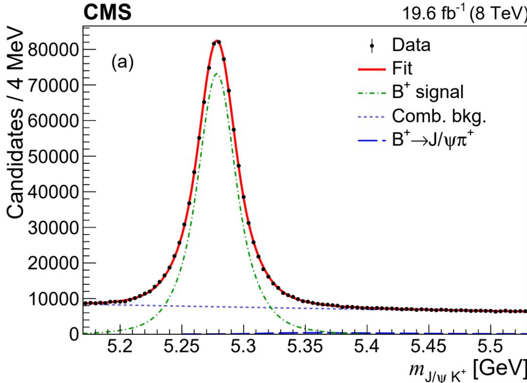
Modelled with triple Gaussian function with common mean for signal, exponential for bkg
