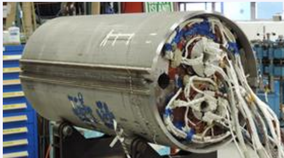
1 meter long Nb_3Sn magnet successfully tested at Fermilab to 11.6T
