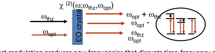
Fast modulation produces new frequencies that disrupts time-frequency chirp
