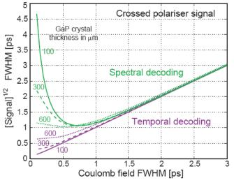
$\tau_{\rm lim} = 2.61 \sqrt{T_0 T_c}$ ; for a Gaussian pulse
