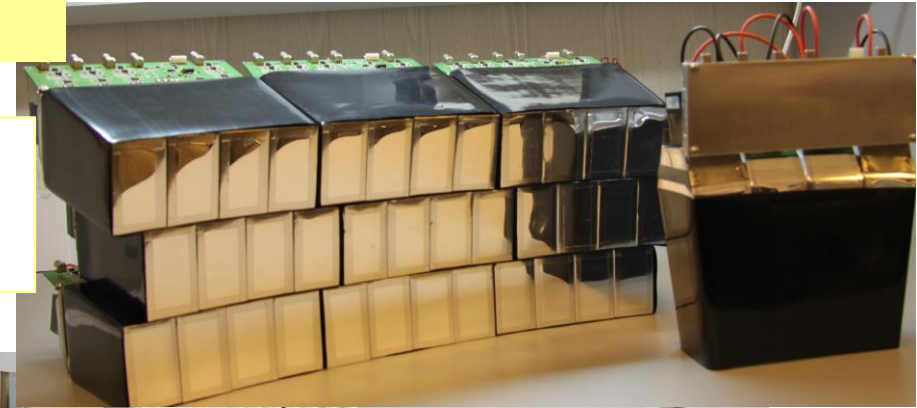
CsI(Tl)/PMT array GADAST (64 units) Energy & position
