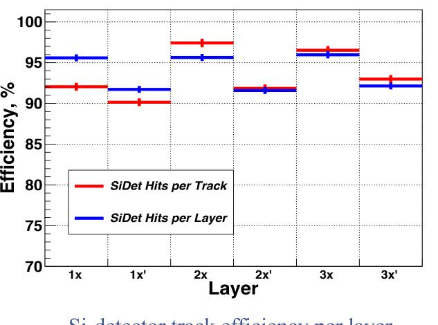
Si-detector track efficiency per layer (using beam trigger)
