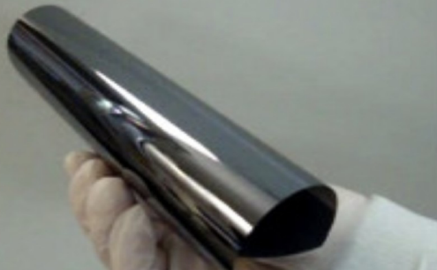
Ultra-thin chip (<50 um): flexible with good stability
