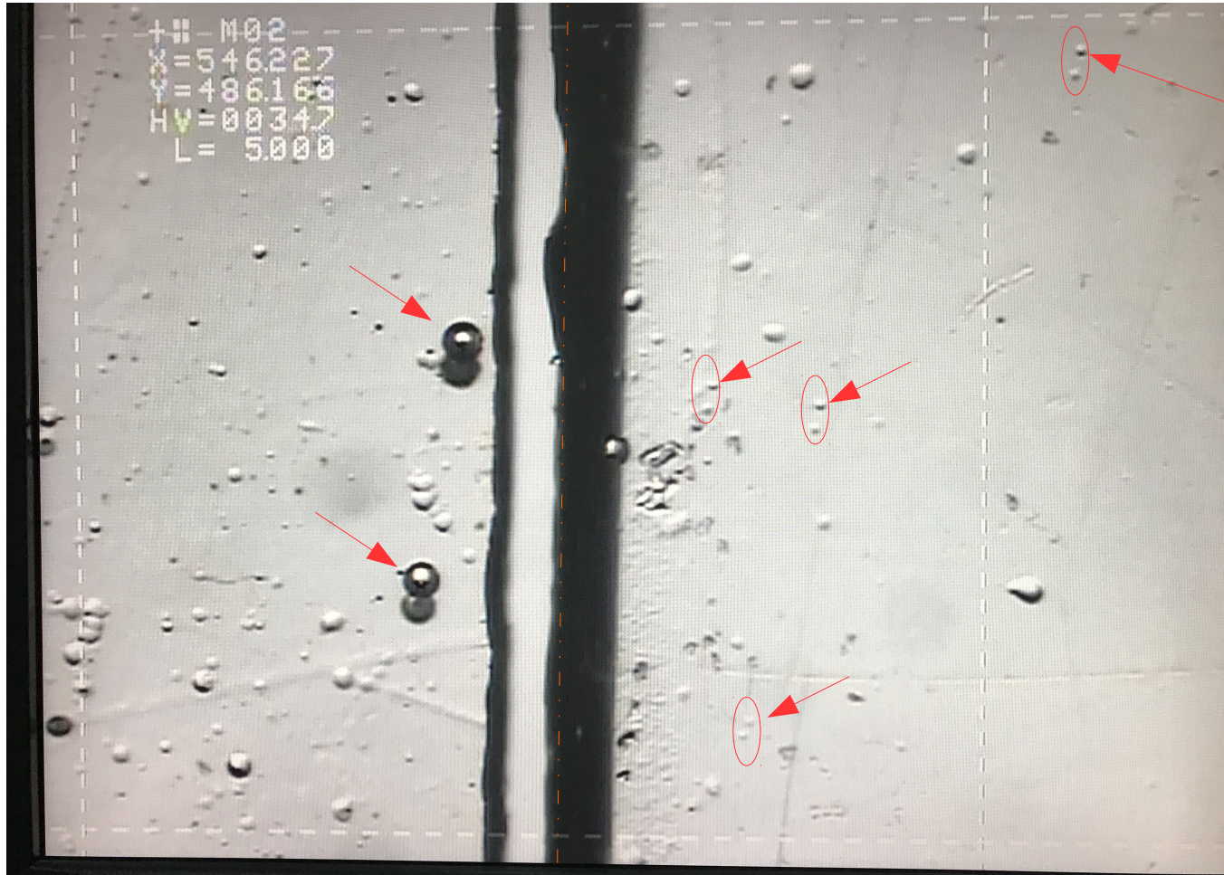
Makrofol exposed to Xe beam, no LHC Previous etchant.
