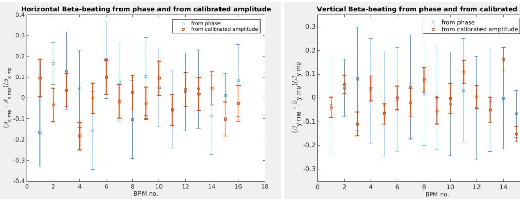
Vertical Beta-beating from phase and from calibrated amplitude
