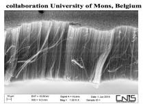
length:  $100 \mu m$  (can be increased) ext. diameter:  $(20 \pm 4) nm$  aspect ratio:  $5x10^4$
