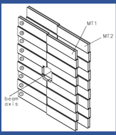
Maximum size of Bakelite electrodes  $\rightarrow$  300 × 180 cm<sup>2</sup>
