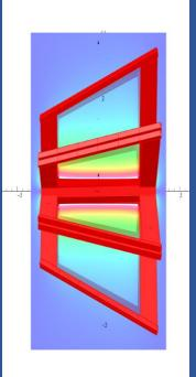
**Open toroid** with field circling the beam axis L = 3m0.3 < R < 1.65 m at entrance 0.3 < R < 2.95 m at exit  $B \cdot R \sim 0.2$ -0.25 Tm
