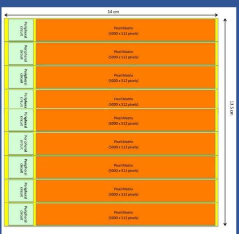
Periphery contains the control logic, the interfaces for the configuration of the chip and the serial data transmitters
