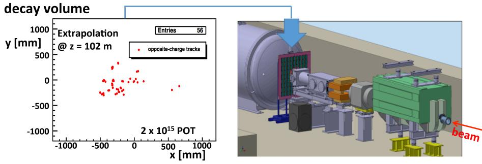
Can be instrumented with a scintillator hodoscope with  $\sigma_T < ^\sim 1$  ns and inefficiency to MIPs  $^\sim 10^{-4}$ , to provide full background rejection at  $10^{18}$  POT Prototype work ongoing
