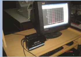
Optical Emission Spectrometer (VS140) and Recorded Spectra
