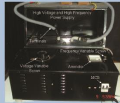
High Voltage and High Frequency Power Supply
