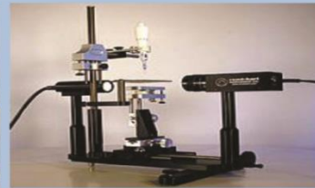
Goniometer for Measurement of Contact Angle
