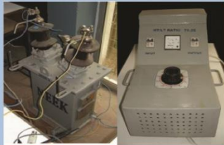
Step up Transformer Which Gives 78.26 Time of the Input Voltage
