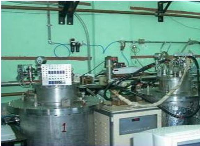
Cryogenic test facility to test corrector magnets at RRCAT
