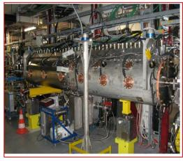
Two Cu coated SS WR 2300 waveguide power couplers installed in the DTL/CCDL in LINAC 4 tunnel at CERN
