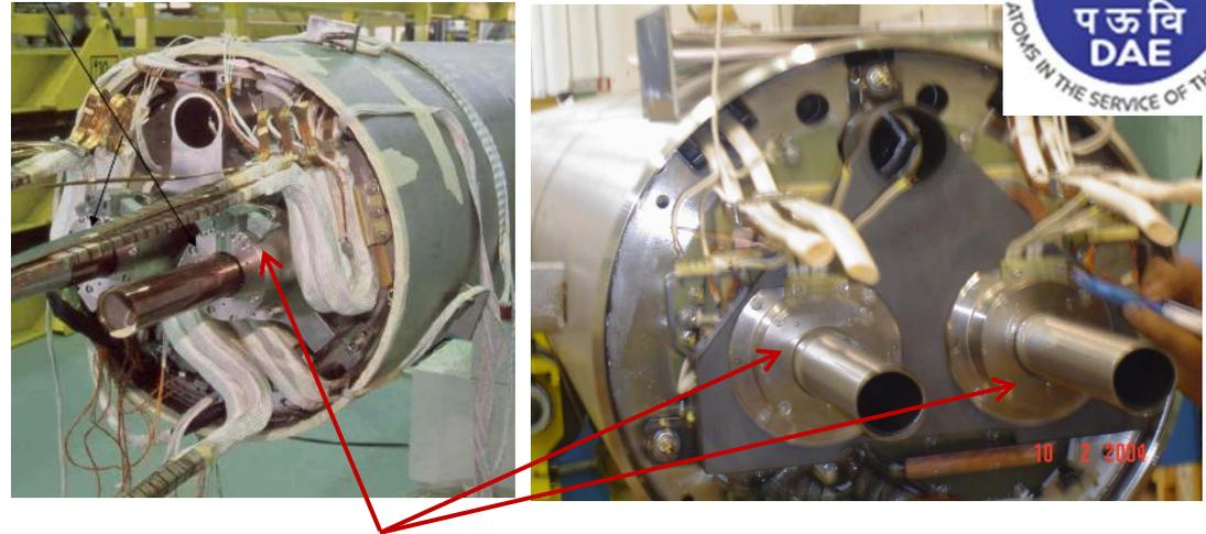
Corrector magnets installed in LHC dipole magnets
