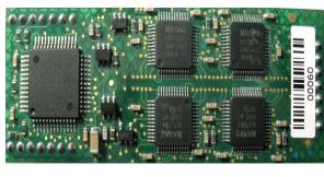
Packaged dimension -7 mm X 7 mm Analog-Digital Chip -  $\sim 6$ , 000 Transistors 16 channel readout
