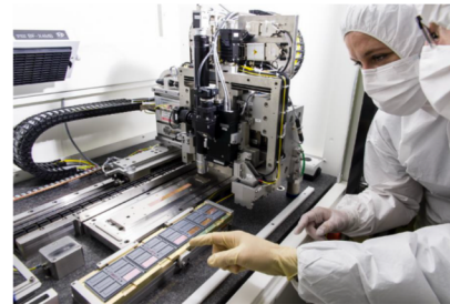
Chip alignment/gluing with ALICIA7 machine
