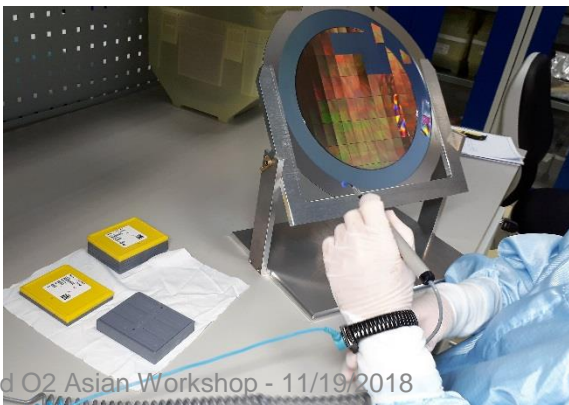
Visual inspection and cleaning
