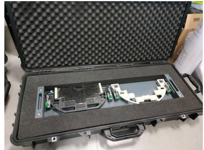
Disk transport tooling for Disk 00/01 and 02
