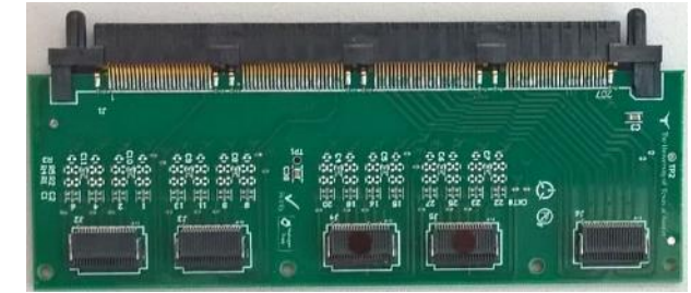
Transition Board v1.0 – compatible with RUv1.x and HDR-192157 cables (and commercial cables)
