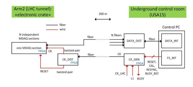
• The BUSY output is set as soon as L1 pulse is received; it is then reset by the control PC (via BUSY\_RST line).
