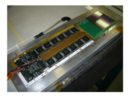
Top side of a Si detector module, showing one Si sensor plane and the corresponding 12 front-end PACE3 chips.
