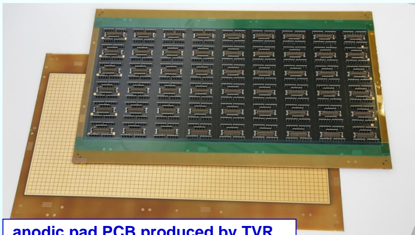
anodic pad PCB produced by TVR
