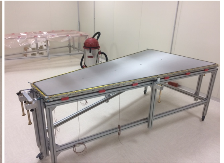
A Completed Drift Panel
