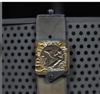
Fixed MgF2 crystal in the vacuum chamber of the coating machine
