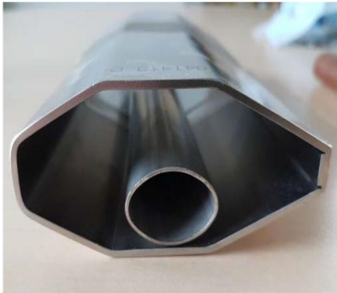
Diamond DDBA upgrade chamber and magnet cross section
