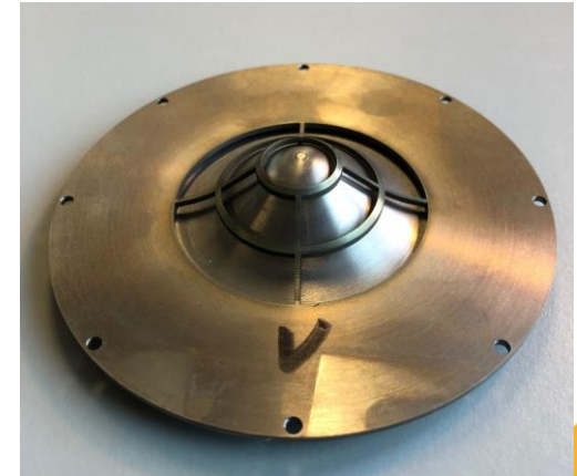
Tungsten prototype for heat load tests
