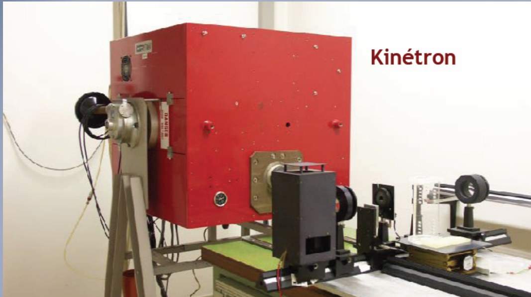
Mounting - Dose distribution with 4.5MeV electrons
