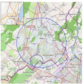
Accelerator complex is located between France and Switzerland. LHC uses the 27 km circumference circular tunnel. The tunnel is located 100 metres underground.
