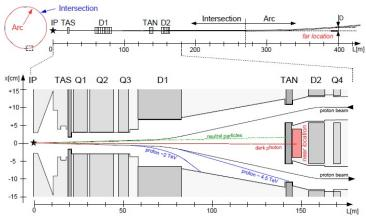
Schematic drawings of the LHC ring and the current very forward infrastructure downstream from the ATLAS and CMS interaction points, along with the representative far and near on-axis detector locations for FASER.
