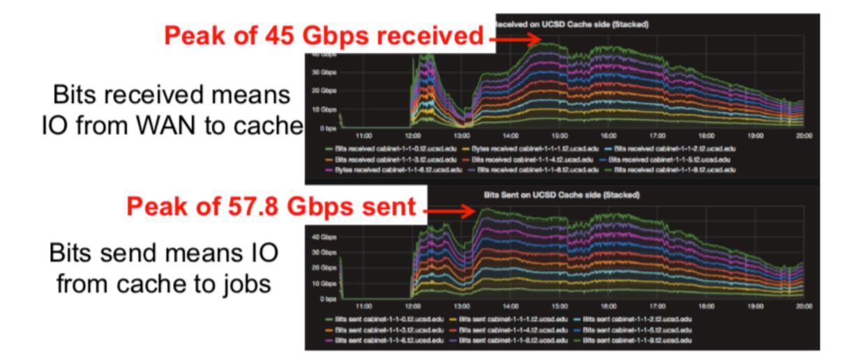
Bits read from disk cache = Bits send – Bits received
