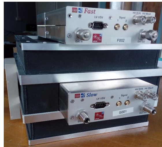
Assembly of a fast and a slow detector size ≈ 20 x 25 x 25 cm 3 (~14 kg)
