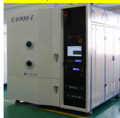
Vacuum chamber for evaporation
