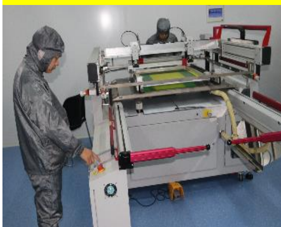
Screen printing with 0.2 mm accuracy for pattern
