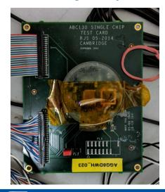
Test card, with connection to the driver board.
