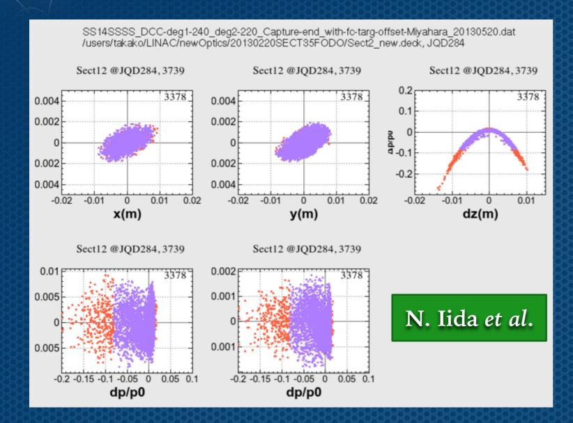
The purple particles are safely injected into the DR. The orange particles are cut by the collimators at LTR because they can not enter the separatrix of DR.
