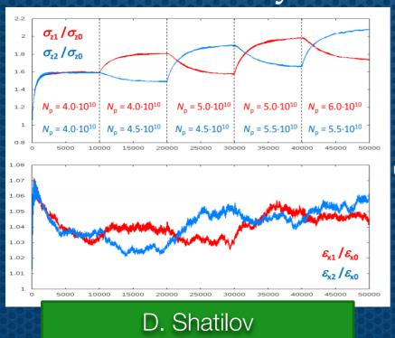
→ Bootstrapping of the charges while topping up in order to control bunch lengthening and emittance fluctuations due to beamstrahlung.
