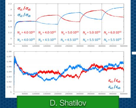
Bootstrapping of the charges while topping up in order to control bunch lengthening and emittance fluctuations due to beamstrahlung.
