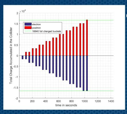
→ Interleaved injection of species in the collider with pre-compensation of the charge loss due to collisions till next round. PS: the full charge is taken as 1.
