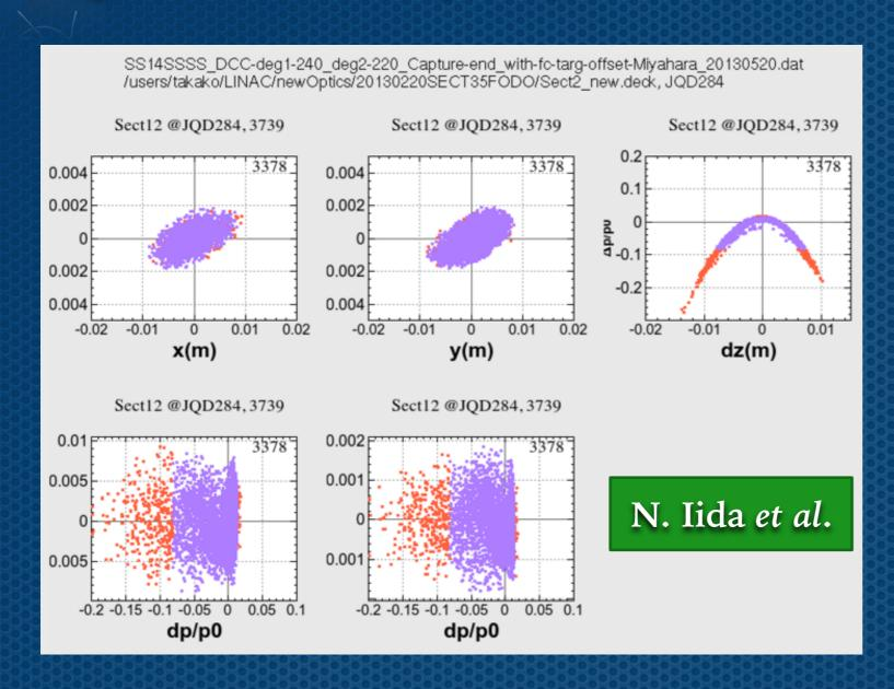
The purple particles are safely injected into the DR. The orange particles are cut by the collimators at LTR because they can not enter the separatrix of DR.
