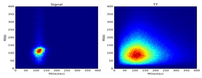
Mass window is optimized Accordingly to the resolution and mean value of m\_tautau and m\_bb distributions:
