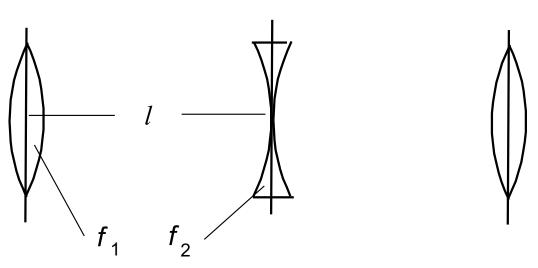
(b) A FODO cell (from mid-F, through D and to the mid-point of the next F) may be considered to be one such matrix with  $f_1 = +2f$  and  $f_2 = -2f$  followed (and multiplied) by another matrix with  $f_1 = -2f$  and  $f_2 = +2f$ . Using the result of the last question, write down these two matrices and show by taking their product that the matrix for a FODO cell from mid-F to mid-F quadrupole is
