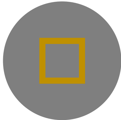
2. Kapton tape which recreates a shape a little smaller than the external dimensions of the chip
