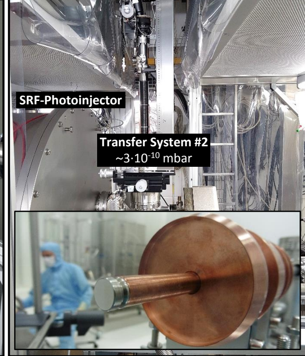
Transfer system #2 at the SRF-photoinjector module
