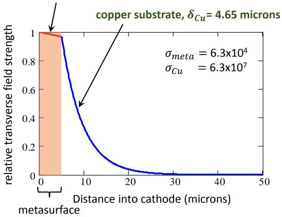
As an example, assume the LCLS-II RF gun frequency of 186 MHz. Using the 6.3x10<sup>4</sup> S/m conductivity of the optimized wire array gives a skin depth of 147 microns. Thus, the RF passes through the 1-micron tall wire array with little dissipation with most of the power being deposited in the higher conductivity metal below with a much shorter skin depth of 4.65 microns.
