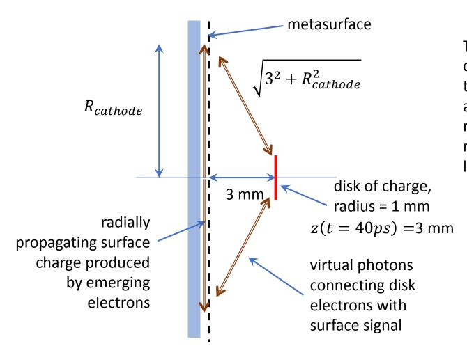
The time it takes a signal to travel from center to edge of cathode and back to disk should longer than the time it takes the image-charge field to decay. That way the signal dies away before the disk can know about the cathode's finite radius. In our example, if the signal velocity is c, then the round-trip distance needs to be longer than the distance light travels in 40 ps, or ct = 12mm. Therefore
