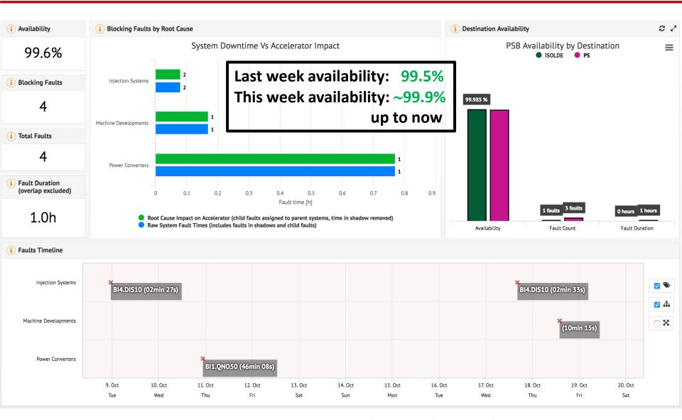
Excellent running last 2 weeks with only a hand-full short faults; a few non-blocking faults of the Finemet cavity degraded R4 intensity for ISOLDE during that period
