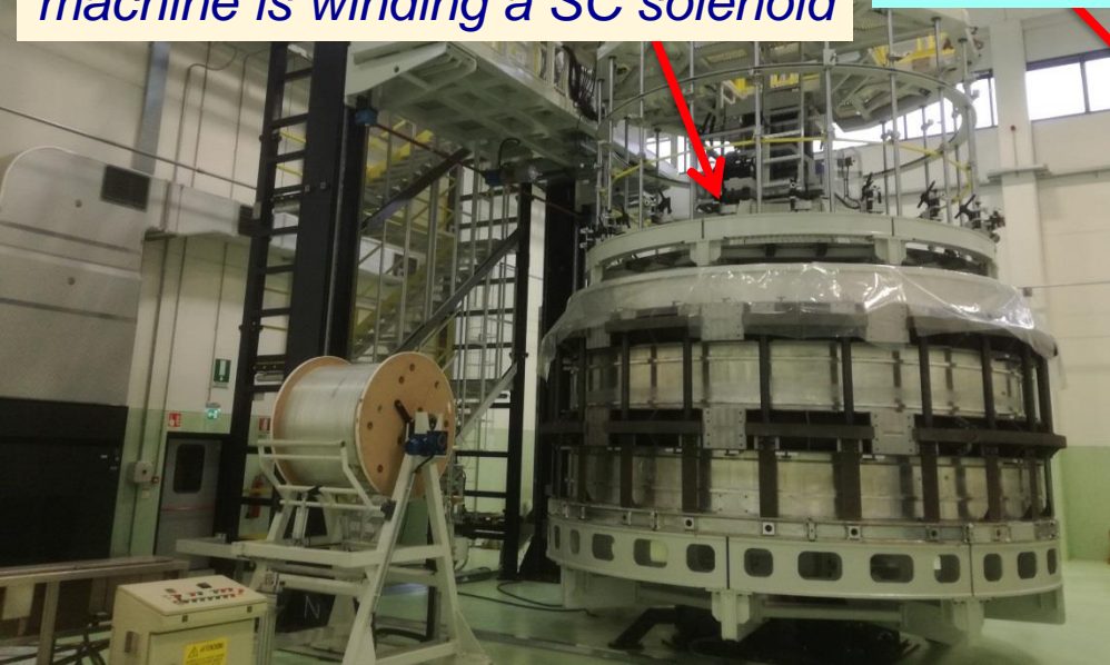
machine is winding a SC solenoid
